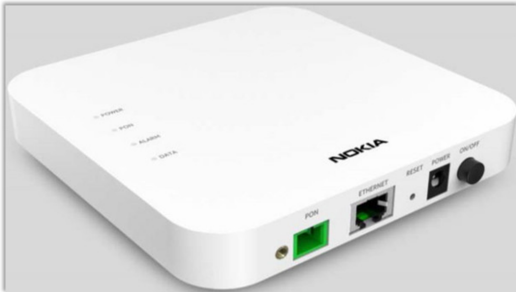
Figure 3: NBI Optical Network Terminal (Nokia XS-010X-Q)
